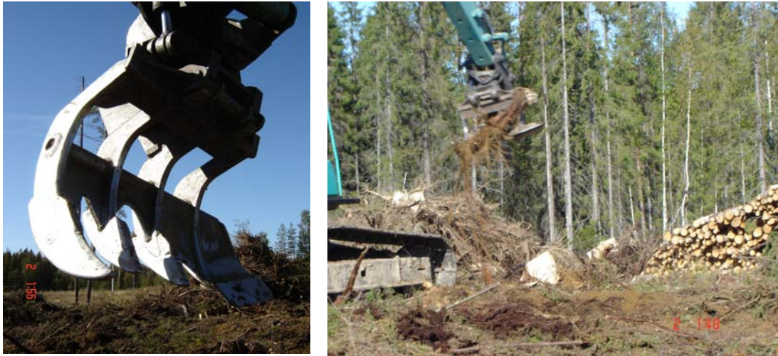
Fig. 3. Stump excavator (left) and stump recovery (right).
