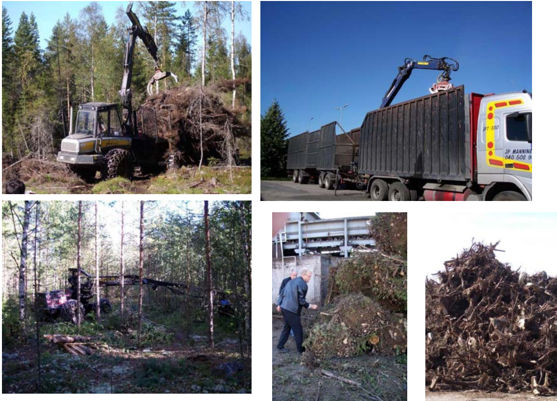
Fig. 2. Forest harvest residue recovery (upper left), residue/stump tandem van with self contained loader and variable size rear compartment (upper right), forest thinning machine (lower left), forest harvest residue “logs” (lower center) and piled dry stumps (lower right).
